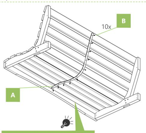
Start mounting the steel flat bar from the 2nd slat from the bottom (see step2 – slat no. 2). Adjust it to the profile of the bench by bending it.
